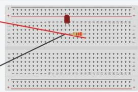
If you connect the longest leg of the LED to a digital pin, You can control it. At this time we connect it to the 9th digital pin to control it.
